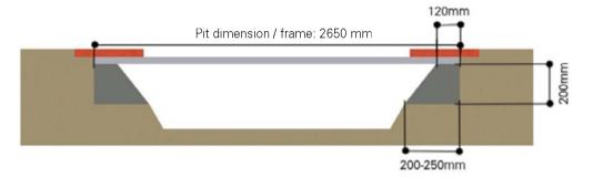
**Attention:** the trampoline may only be installed on a flat surface and under no circumstances on a mound, incline or slope edge.
